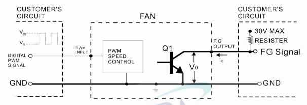
\*TRANSISTOR Q1 AT "ON" POSITION
