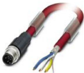
Bus system cable, CC link (10 Mbps), 4-position, PVC, red, shielded, Plug straight M12, coding: A, on free cable end, cable length: 2 m
