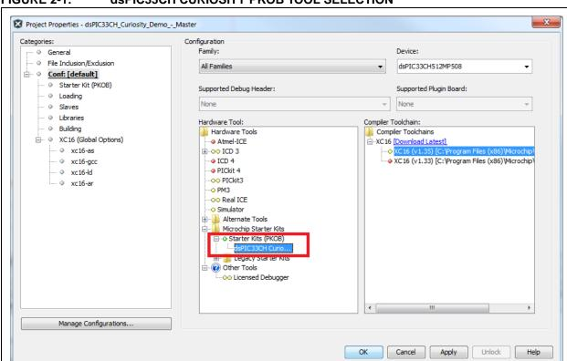
FIGURE 2-1: dsPIC33CH CURIOSITY PKOB TOOL SELECTION
