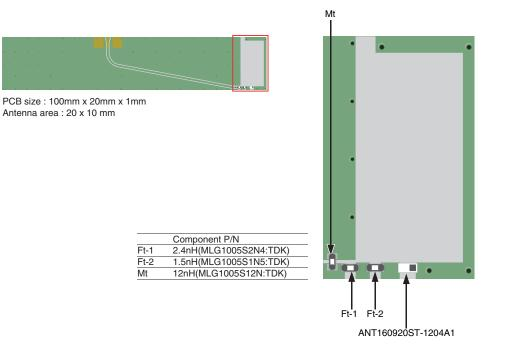
□Measurement condition for Radiation Pattern
