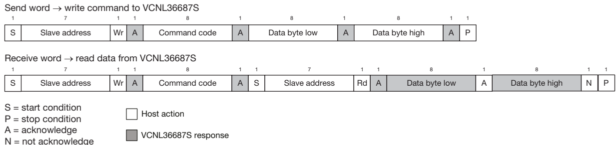
Fig. 9 - Write Word and Read Word Protocol
