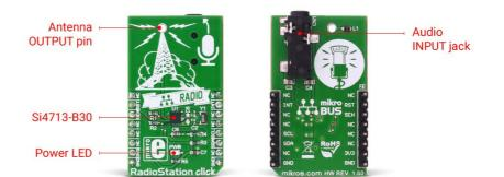
The click is designed for communication over the I2C/2-wire control interface. When selecting 2-wire mode, SCLK pin should stay at a HIGH logic level during the rising edge on the RST pin, and stay HIGH until after the first start condition. Also, a start condition must not occur within 300nS before the rising edge on the RST pin. The 2-wire bus mode uses only the SCL and SDA pins for communication.
