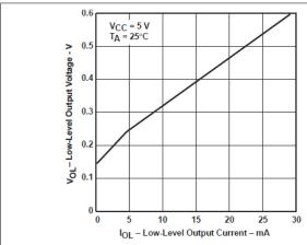
Figure 5-7. Receiver Low-Level Output Voltage vs Low-Level Output Current
