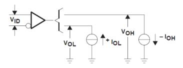
Figure 6-2. Receiver  $V_{OH}$  and  $V_{OL}$
