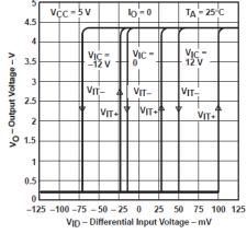
Figure 5-3. Driver Differential Output Voltage vs Output Current | Figure 5-4. Receiver Output Voltage vs Differential Input Voltage
