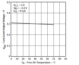
Figure 5-8. Receiver Low-Level Output Voltage vs Free-Air Temperature
