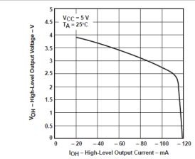
Figure 5-1. Driver High-Level Output Voltage vs High-Level **Output Current**
