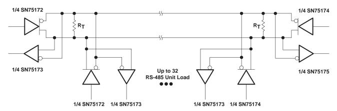
NOTE A: The line length should be terminated at both ends in its characteristic impedance (R<sub>T</sub> = Z<sub>O</sub>). Stub lengths off the main line should be kept as short as possible.
