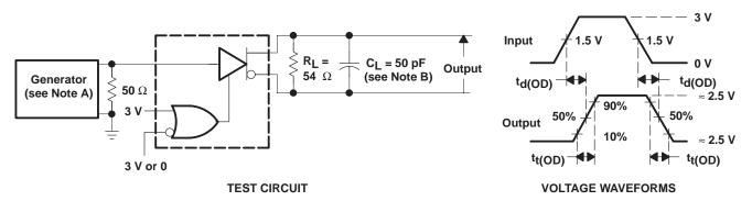
NOTES: A. The input pulse is supplied by a generator having the following characteristics:  $t_f \le 5$  ns,  $t_f \le 5$  ns,  $t_f \le 5$  ns, PRR  $\le 1$  MHz, duty cycle = 50%,  $t_f \le 5$  ns,  $t_$
