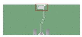
PCB size: 50mm x 10mm x 1mm Antenna area : 5 x 3 mm
