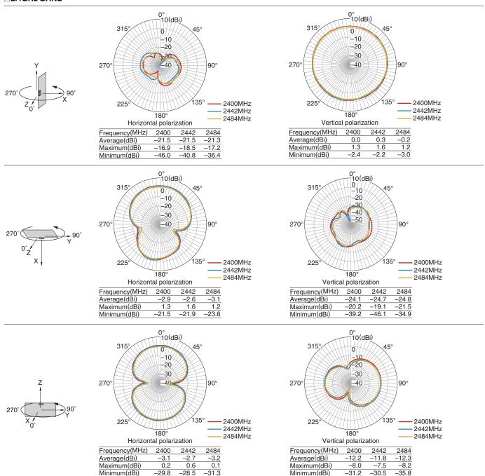
• Tested antenna has been soldered. Evaluation board size is 50×20×1 mm.
