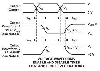
NOTES: A. C<sub>1</sub> includes probe and jig capacitance.
