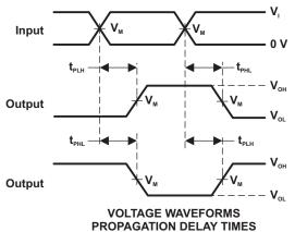
INVERTING AND NONINVERTING OUTPUTS
