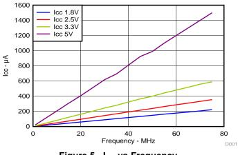
Figure 5. I<sub>CC</sub> vs Frequency
