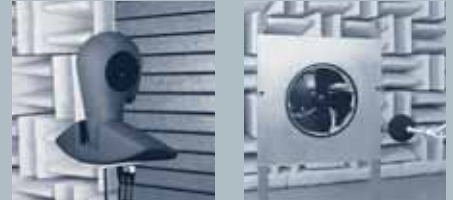
Room for precision noise measuring
