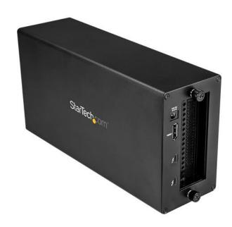
This Thunderbolt<sup>™</sup>3 PCIe expansion chassis lets you add a PCI Express card to your laptop or desktop computer, through an external Thunderbolt 3 connection. The chassis also features a DisplayPort video output, so you can connect an additional monitor to your laptop, and supports Thunderbolt 3 daisy chaining, so you can expand your workstation even further.
