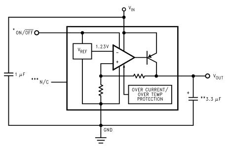
$<sup>^{\</sup>star}$ ON/ $\overline{\text{OFF}}$  input must be actively terminated. Tie to  $V_{\text{IN}}$  if this function is not to be used.
