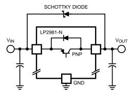
Figure 39. Adding External Schottky Diode Protection
