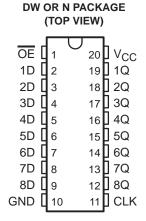
The eight flip-flops of the SN74F574 are edge-triggered D-type flip-flops. On the positive transition of the clock (CLK) input, the Q outputs will be set to the logic levels that were set up at the data (D) inputs.
