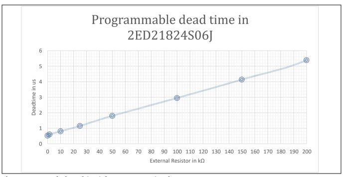
Figure 11 Variation of dead time vs. external resistor
