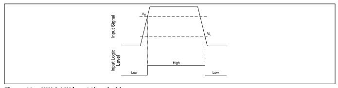
Figure 12 HIN & LIN input thresholds
