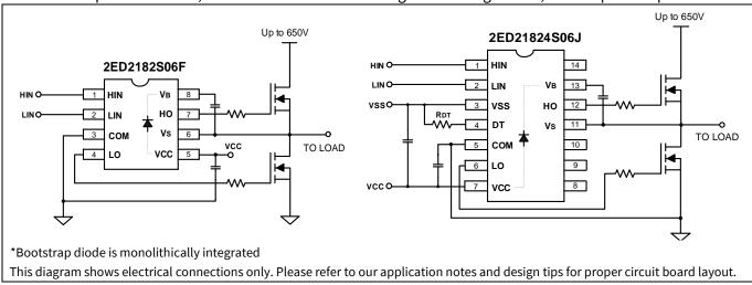
Figure 1 Typical application block diagram
