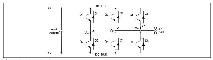
Figure 18 Three phase inverter
