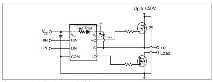
Figure 16 Half bridge bootstrap circuit in 2ED218x
