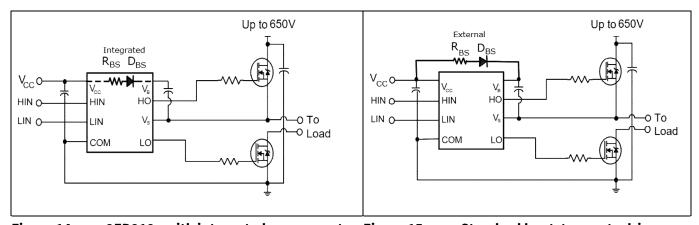
Figure 14 2ED218x with integrated components Figure 15 Standard bootstrap gate driver
