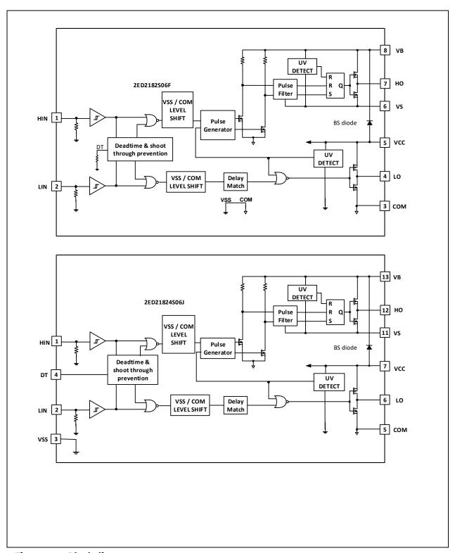
Figure 2 Block diagrams
