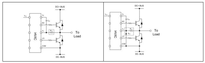
Figure 25 Resistor between the VS pin and the switch node
