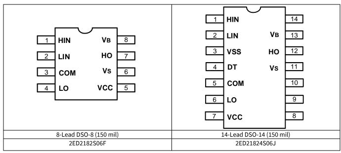
Figure 3 2ED2182(4)S06F(J) pin assignments (top view)
