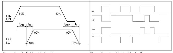
Figure 6 Switching timing diagram
