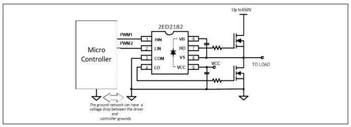
Figure 17 Negative voltage tolerance on inputs of upto -5 V
