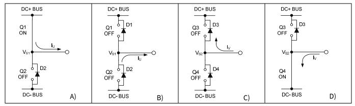
Figure 19 A) Q1 conducting B) D2 conducting C) D3 conducting D) Q4 conducting
