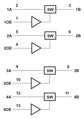
Figure 2. Logic Diagram (Positive Logic)
