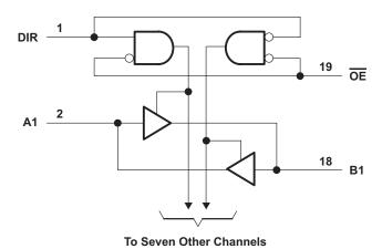
Figure 3. Logic Diagram (Positive Logic)
