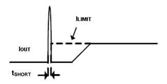
Figure 2. Response Time to Short-Circuit Waveform
