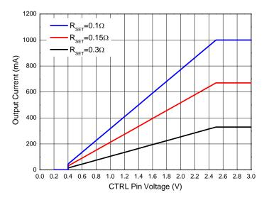
Figure 1. Analog Dimming Curve
