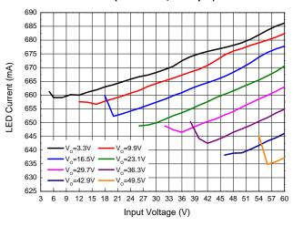
LED Current vs. Input Voltage (R<sub>S</sub>=0.1Ω, L=100μH)
