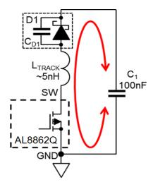
Figure 3. PCB Loop Resonance
