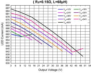
LED Current vs. Output Voltage
