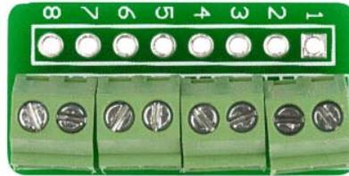
PROTO Connect board provides a convenient way of connecting eight wires from power supply, communication, analog or GPIO lines to the target breadboard. Board features eight screw terminals and eight connection pads in standard 100mil distance. Board is compact and cheap thus making it a good choice for prototyping.
