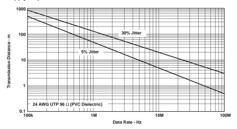
Figure 21. Data Transmission Distance Versus Rate
