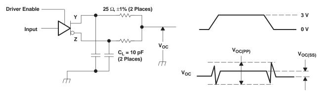
A. All input pulses are supplied by a generator having the following characteristics:  $t_r$  or  $t_r \le 1$  ns, pulse repetition rate (PRR) = 50 Mpps, pulse width =  $10 \pm 0.2$  ns .  $C_L$  includes instrumentation and fixture capacitance within 0,06 mm of the D.U.T. The measurement of  $V_{OC(PP)}$  is made on test equipment with a -3 dB bandwidth of at least 300 MHz.
