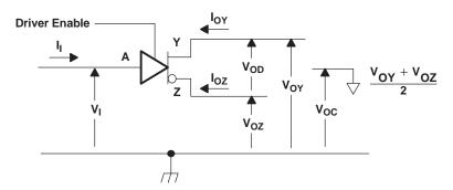
Figure 1. Driver Voltage and Current Definitions
