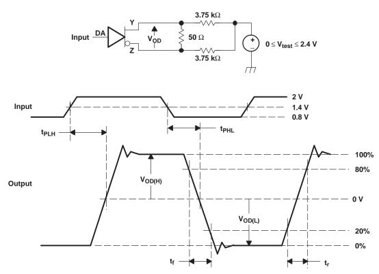
A. All input pulses are supplied by a generator having the following characteristics:  $t_r$  or  $t_r \le 1$  ns, pulse repetition rate (PRR) = 50 Mpps, pulse width =  $10 \pm 0.2$  ns .  $C_L$  includes instrumentation and fixture capacitance within 0,06 mm of the D.U.T.
