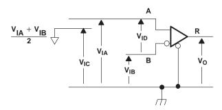
Figure 5. Receiver Voltage Definitions
