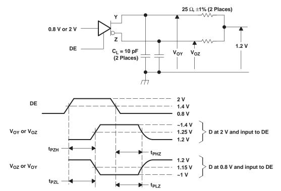
A. All input pulses are supplied by a generator having the following characteristics:  $t_r$  or  $t_t \le 1$  ns, pulse repetition rate (PRR) = 0.5 Mpps, pulse width = 500 ± 10 ns .  $C_L$  includes instrumentation and fixture capacitance within 0,06 mm of the D.U.T.
