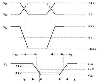
A. All input pulses are supplied by a generator having the following characteristics:  $t_r$  or  $t_l \le 1$  ns, pulse repetition rate (PRR) = 50 Mpps, pulse width = 10  $\pm$  0.2 ns.  $C_L$  includes instrumentation and fixture capacitance within 0,06 mm of the D.U.T.
