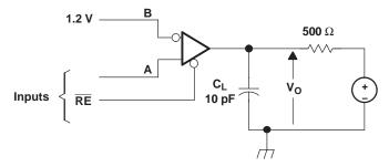
NOTE A: All input pulses are supplied by a generator having the following characteristics:  $t_r$  or  $t_f \le 1$  ns, pulse repetition rate (PRR) = 0.5 Mpps, pulse width =  $500 \pm 10$  ns.  $C_L$  includes instrumentation and fixture capacitance within 0,06 mm of the D.U.T.
