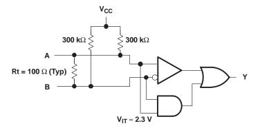
Figure 22. Open-Circuit Fail Safe of the LVDS Receiver
