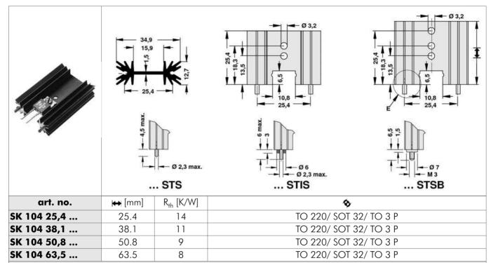
STIS =with solder pins and insulating washer
