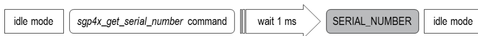
Figure 10 Process flow for reading out the serial number of the SGP40 sensor.
