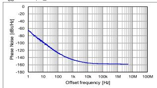
Phase Jitter (Offset frequency: 12 kHz to 5 MHz)
