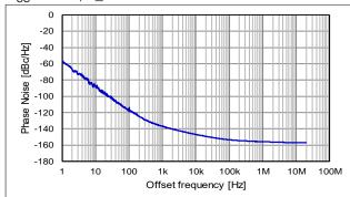
Phase Jitter (Offset frequency: 12 kHz to 20 MHz)
