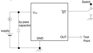
\*Standby current test should be  $\overline{ST} = GND$ .
