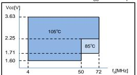
Please note that Supply voltage range ( $V_{CC}$ ) depends on Output frequency(fo) and upper limit of Operating temperature( $T_{use}$  Max.).
