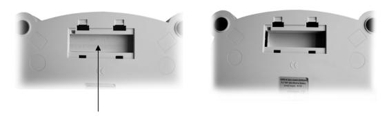
2. Slide spacer to left or right, lever down on corner, then remove the spacer
