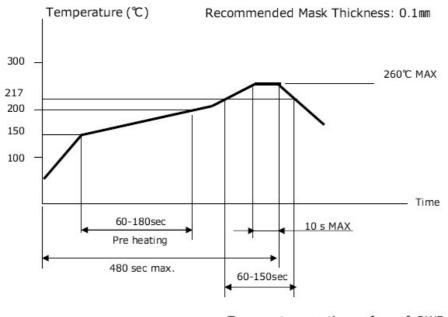
Temperature on the surface of PWB
