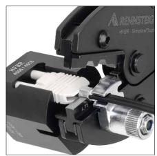
Ultra-precise plug positioning with special 3x positioning guide and locking clamp aid
