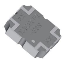
The X3C26P1-30S is a low profile, high performance 30dB directional coupler in a new easy to use, manufacturing friendly surface mount package. It is designed for WIMAX and LTE band applications. The X3C26P1-30S is designed particularly for power and frequency detection, as well as for VSWR monitoring, where tightly controlled coupling and low insertion loss is required. It can be used in high power applications up to 200 Watts.
