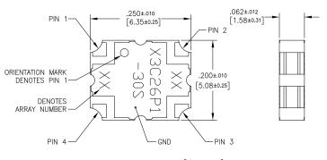
Dimensions are in Inches [Millimeters] X3C26P1-30S Mechanical Outline
