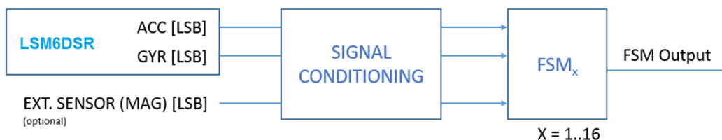
Figure 2. State machine in the LSM6DSR
