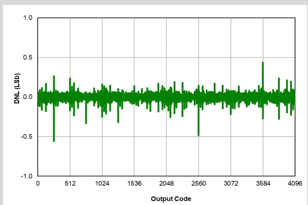
Figure 40-48. ADC 12-Bit Mode, Single-Ended Typical DNL, V DD = 3.0V, V REF = 3.0V, T AD = 0.5 μs, 25°C, All devices
