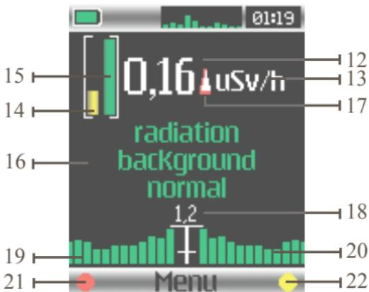
12. Radioactivity level. The radioactivity level is shown with large figures in the center of the screen. When the device is taking measurements for the first time, the word «Measurement» appears on the screen.
