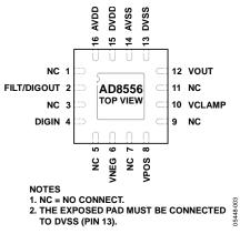
Figure 3. 16-Lead LFCSP\_WQ Pin Configuration
