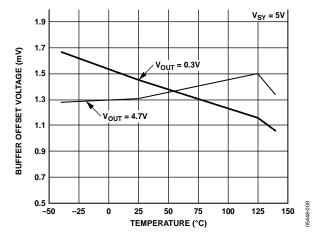
Figure 8. Output Buffer Offset Voltage vs. Temperature
