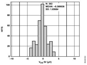
Figure 4. Input Offset Voltage Distribution
