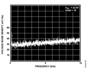
FREQUENCY (kHz) Figure 19. Voltage Noise Density vs. Frequency (0 Hz to 10 kHz)
