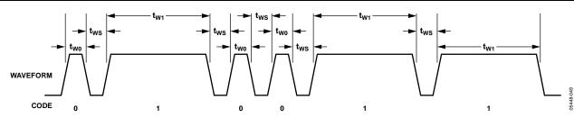
Figure 49. Timing Diagram for Code 010011
