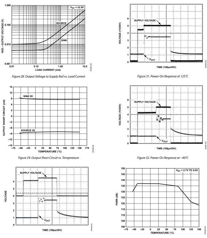
Figure 30. Power-On Response at 25°C
