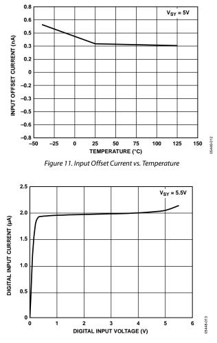
Figure 12. Digital Input Current vs. Digital Input Voltage (Pin 4)
