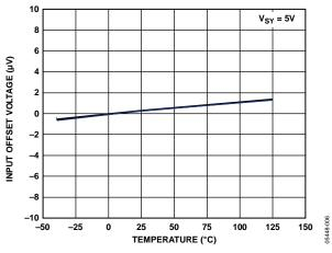
Figure 6. Input Offset Voltage vs. Temperature
