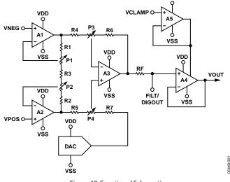
Figure 47. Functional Schematic
