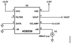
Figure 54. Test Circuit to Show AD8556 Performance Exposed to Differential Mode RFI/EMI Signals
