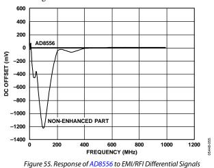
To make a board robust against EMI, the leads at VPOS and VNEG should be as similar as possible. In this way, any EMI received by the VPOS and VNEG pins will be similar (that is, a common-mode input), and rejected by the AD8556. Furthermore, additional filtering at the VPOS and VNEG pins should give a better reduction of unwanted behavior compared with filtering at the other pins.
