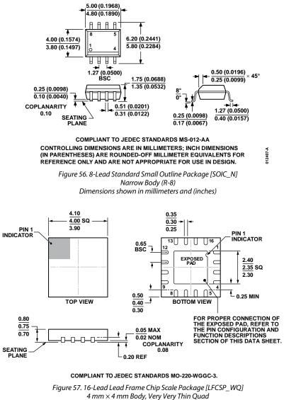
4 mm × 4 mm Body, Very Very Thin Quae (CP-16-20) Dimensions shown in millimeters
