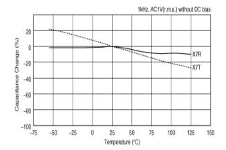
Capacitance - temperature characteristics
