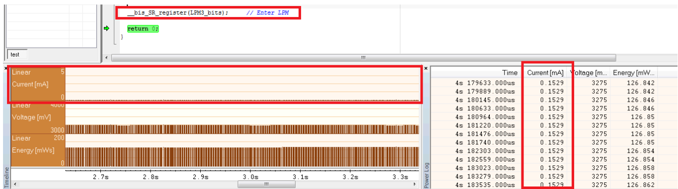
Figure 3-19. LPM3 Current When Executing Under Debug Control
