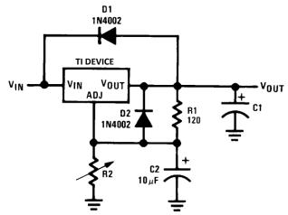
$\begin{aligned} & \text{Copyright} \circledcirc 2016, \, \text{Texas Instruments Incorporated} \\ & V_{OUT} = 1.25V \left(1 + \frac{R2}{R1}\right) + I_{ADJ}R2 \end{aligned}$
