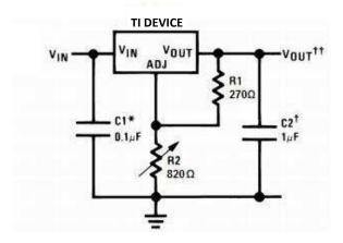
\*Needed if device is more than 6 inches from filter capacitors.
