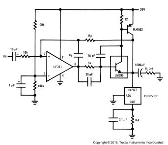
$A_V = 1$ ,  $R_F = 10k$ ,  $C_F = 100 pF$  $A_V = 10$ ,  $R_F = 100k$ ,  $C_F = 10 pF$
