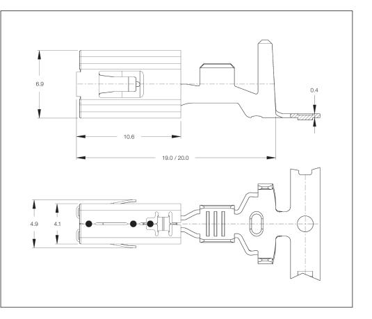
Mating Force: max. 16 N Unmating Force: max. 11 N Extraction Tool: Part No. 1-1579007-3
