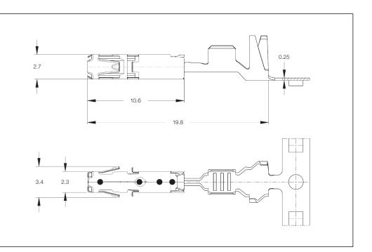
$\label{eq:contact Resistance:} \begin{array}{l} \mbox{New State} \leq 2 \ m\Omega \end{array} \\ \mbox{Mating Force:} \\ \mbox{Max. 6 N} \\ \mbox{Unmating Force:} \\ \mbox{Max. 6 N} \end{array}$
