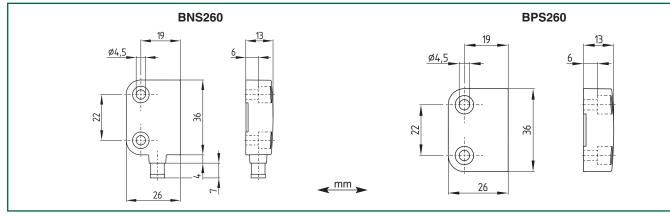
Note: BNS260 reed switch assemblies should be mounted at least 50mm (2") apart.
