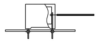
Temperature monitored inside the capacitor.
