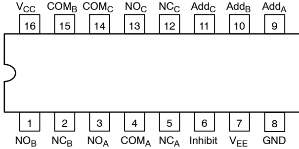
Figure 1. Pin Connection (Top View)
