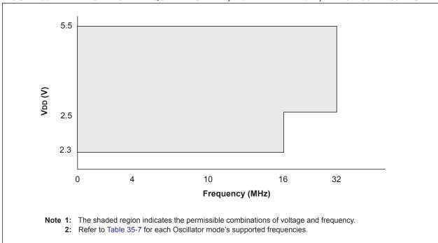
FIGURE 35-2: VOLTAGE FREQUENCY GRAPH, -40°C  $\leq$  Ta  $\leq$  +125°C, PIC16LF18324/18344 ONLY
