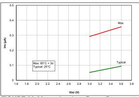
FIGURE 36-20: IPD, Low-Power Brown-out Reset (LPBOR = 0), PIC16LF18324/18344 Only
