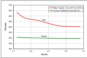
FIGURE 36-114: Wake From Sleep, LFINTOSC, PIC16LF18324/18344 Only
