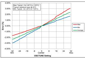
FIGURE 36-104: OSCTUNE Center Frequency, PIC16LF18324/18344 Only
