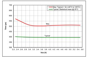
FIGURE 36-113: Wake From Sleep, VREGPM = 1, LFINTOSC, PIC16F18324/18344 Only
