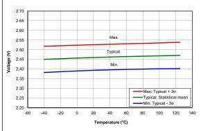
FIGURE 36-43: Brown-out Reset Voltage, Trip Point, (BORV = 1), PIC16F18324/18344 Only
