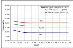
FIGURE 36-30: LFINTOSC Frequency, PIC16F18324/18344 Only
