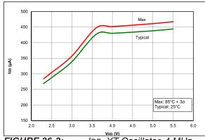
FIGURE 36-2: IDD, XT Oscillator, 4 MHz, PIC16F18324/18344 Only
