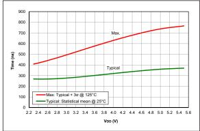
FIGURE 36-89: Comparator Response Time Rising edge, PIC16F18324/18344 Only
