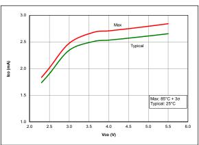
**FIGURE 36-4:** IDD, HS Oscillator, 32 MHz, PIC16F18324/18344 Only
