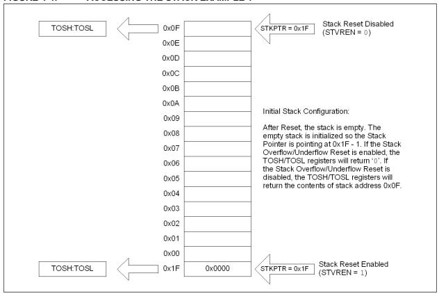
FIGURE 4-5: ACCESSING THE STACK EXAMPLE 2
