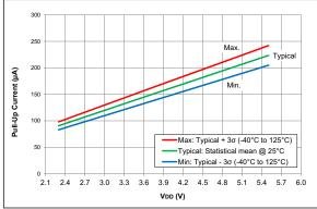
FIGURE 36-31: Weak Pull-Up Current, PIC16F18324/18344 Only
