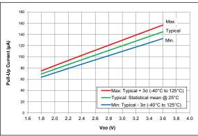
FIGURE 36-32: Weak Pull-Up Current, PIC16LF18324/18344 Only
