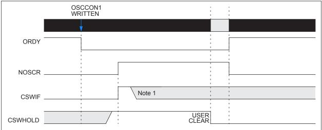
Note 1: CSWIF is asserted coincident with NOSCR, and may be cleared before or after clearing CSWHOLD = 0.
