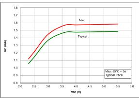
FIGURE 36-8: IDD, HFINTOSC Mode, Fosc = 16 MHz, PIC16F18324/18344 Only
