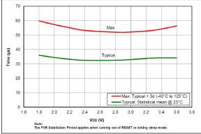
**FIGURE 36-91:** FVR Stabilization Period, PIC16LF18324/18344 Only
