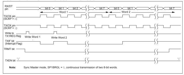
FIGURE 31-11: SYNCHRONOUS TRANSMISSION (THROUGH TXEN)
