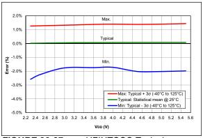
FIGURE 36-27: HFINTOSC Typical Frequency Error, PIC16F18324/18344 Only
