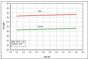
FIGURE 36-22: IPD, Comparator, PIC16LF18324/18344 Only
