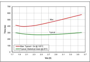
FIGURE 36-88: Comparator Response Time Rising edge, PIC16LF18324/18344 Only
