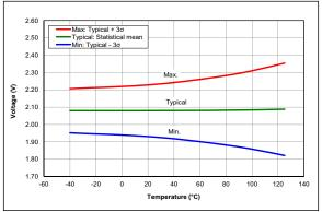
FIGURE 36-45: LPBOR Reset Voltage, PIC16LF18324/18344 Only
