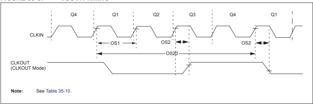
TABLE 35-7: EXTERNAL CLOCK/OSCILLATOR TIMING REQUIREMENTS
