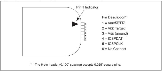
FIGURE 33-3: TYPICAL CONNECTION FOR ICSP™ PROGRAMMING
