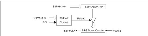
**Note:** Values of 0x00, 0x01 and 0x02 are not valid for SSP1ADD when used as a Baud Rate Generator for I<sup>2</sup>C. This is an implementation limitation.
