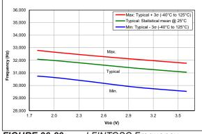
FIGURE 36-29: LFINTOSC Frequency, PIC16LF18324/18344 Only
