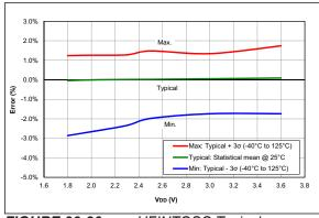
FIGURE 36-26: HFINTOSC Typical Frequency Error, PIC16LF18324/18344 Only
