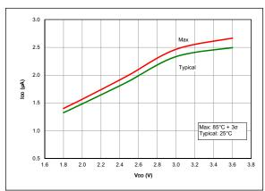
**FIGURE 36-3:** IDD, HS Oscillator, 32 MHz, PIC16LF18324/18344 Only
