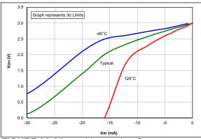
FIGURE 36-35: VOH vs. IOH Over Temperature, VDD = 3.0V, All devices
