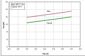
**FIGURE 36-19:** IPD, Brown-out Reset (BOR), BORV = 1, PIC16F18324/18344 Only
