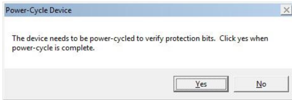
Figure 4.9: Power-cycle required to begin verification.
