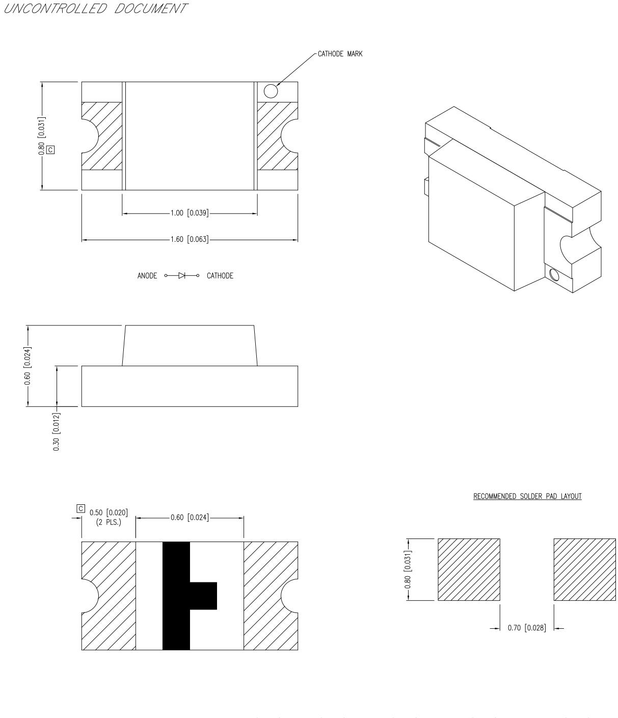
\*UNLESS OTHERWISE SPECIFIED TOLERANCES PER DECIMAL PRECISION ARE: X=±1 (±0.039), X.X=±0.5 (±0.020), X.XX=±0.25 (±0.010), X.XXX=±0.127 (±0.005). LEAD SIZE=±0.05 (±0.030). MIN=  $\frac{+0.00}{-0.00}$  MAX.=  $\frac{+0.00}{-0.00}$  MAX.
