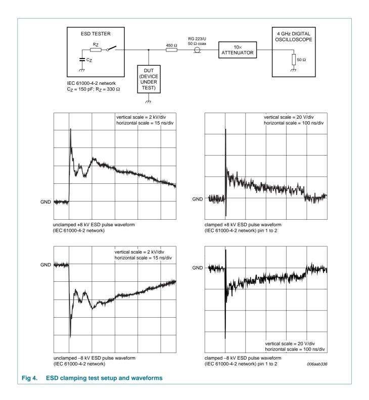
Ultra low capacitance bidirectional ESD protection diodes
