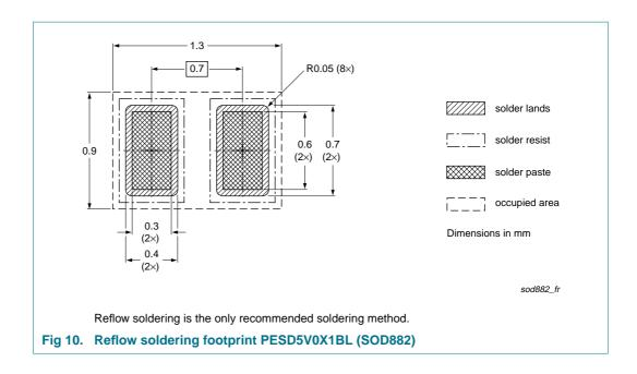
Ultra low capacitance bidirectional ESD protection diodes
