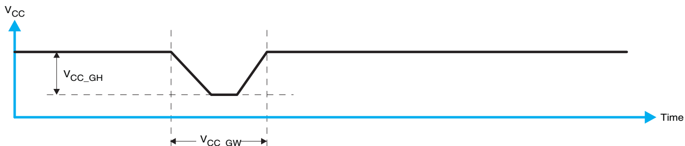
Figure 25. Glitch Width and Glitch Height
