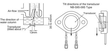
The arrows indicate the tilt direction of the transducer.
