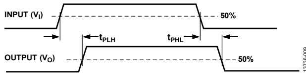
Figure 11. Propagation Delay Parameters
