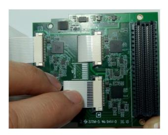
Figure 2. Camera Connection Detail
