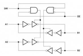
Figure 3. Logic Diagram for SN74AVC4T245
