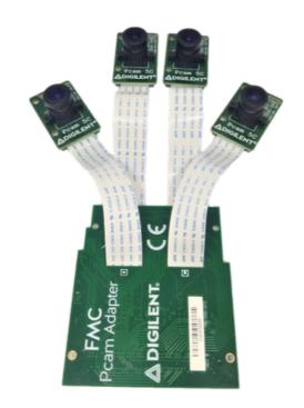
Figure 1. Four Camera Connection
