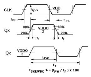
Figure 3. AC Reference Measurement
