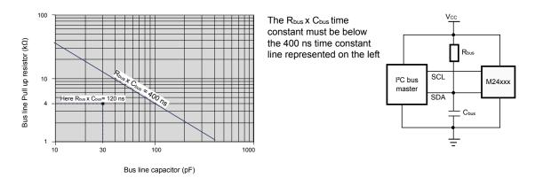
Figure 17. Maximum Rbus value vs. bus parasitic capacitance (Cbus) for an  $I^2C$  bus at  $f_C = 1MHz$
