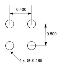
Figure 20. WLCSP4 (CU) - Recommended footprint
