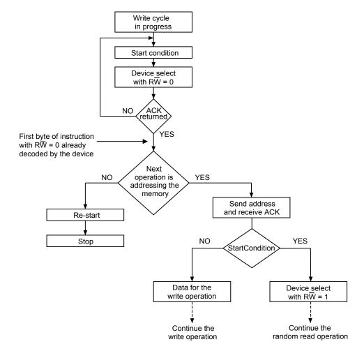
Figure 7. Write cycle polling flowchart using ACK
