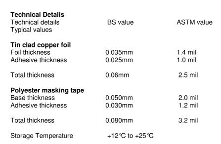
Please also see data sheet for AT536 35 micron Tin Clad Copper Shielding Tape (Unmasked product).
